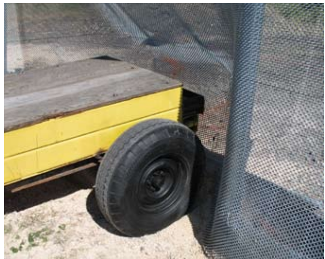
Bogey vehicle weighing 4,000 lbs. and moving 20 mph was stopped in just 4 feet by 1/2" Mesh x 9 GA chain link fence.
